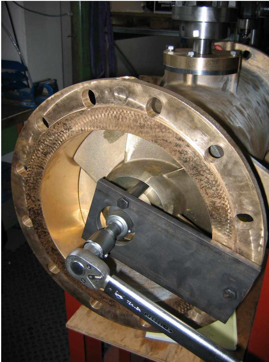
Picture 1: Loosen of impeller nut with help of tools D1.004 bzw. D1.004-1
