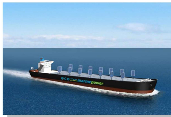
Fig. 6. The Aquarius Eco Ship concept is based on the Energy Sail technology that uses solar panels embedded in rigid sails [22].
