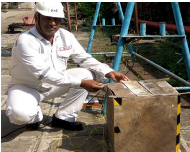
Fig. 3. FRP test cabin top covered
