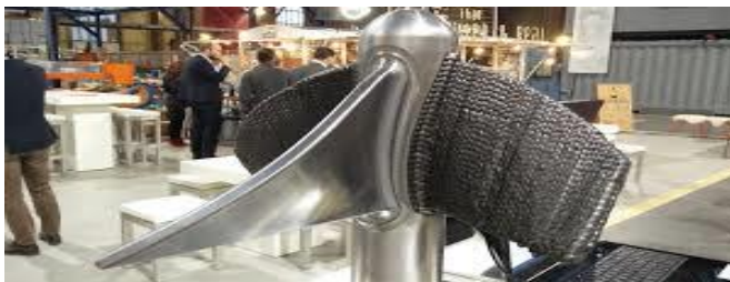
Fig. 3 Picture of a boat propeller better known as WAAMPeller
