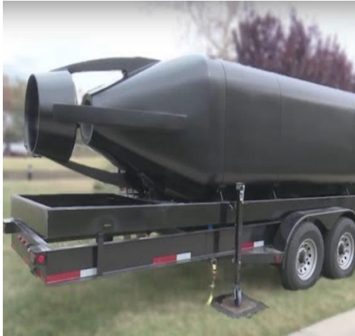
Fig Picture of 3D printed submarine hull prototype by the U.S. Navy
