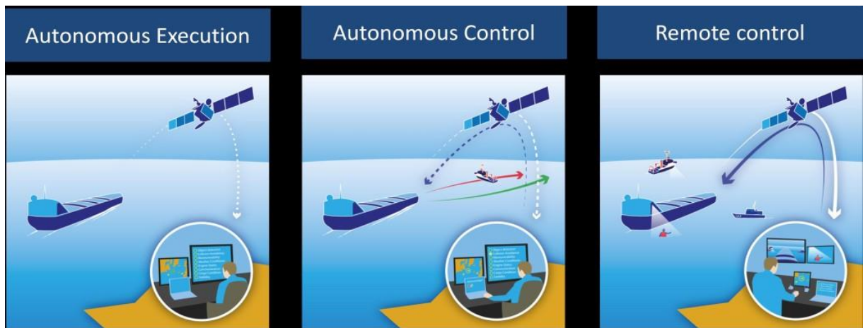
Figure 5.3 Various types of ship navigation for autonomous and remote controlled ship.
