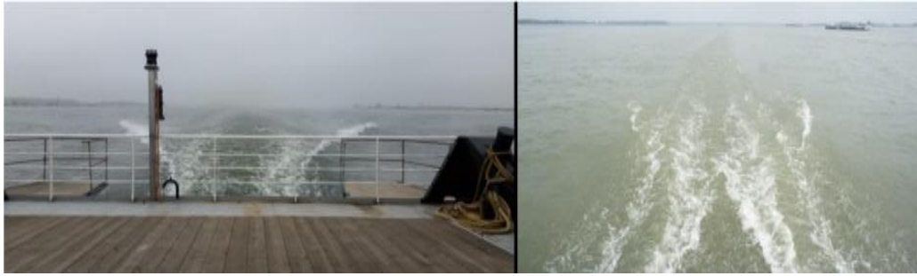
Fig. 7: Comparison of the wave profile of the 55 metre supply vessel without Hull Vane (lefthand) with Hull Vane(right).
