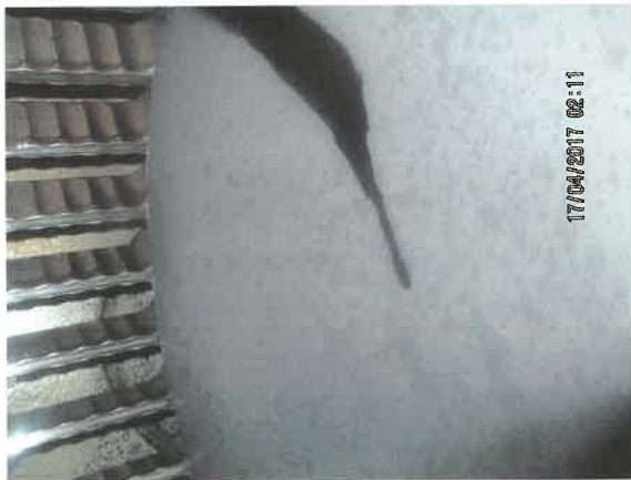
No.3 cyl unit Fuel oil leakage from fuel oil injector on piston crown
