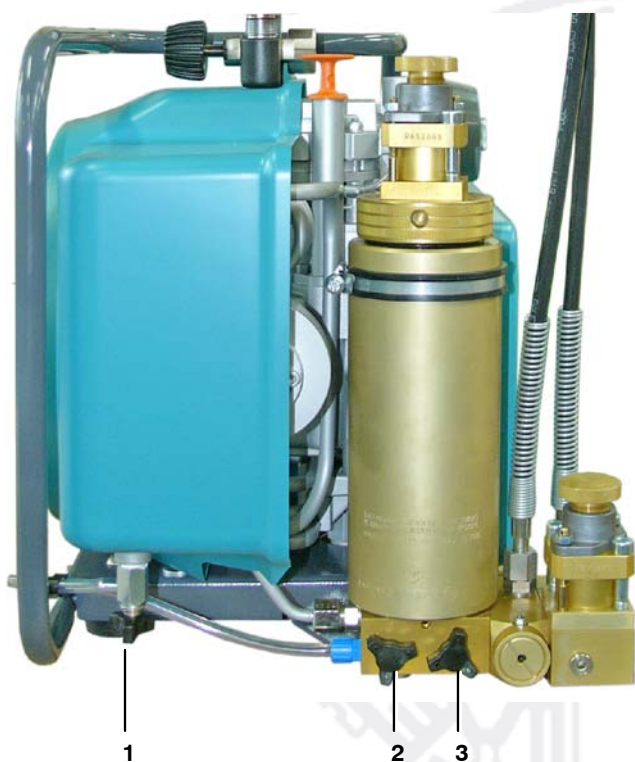
Fig. 28 Condensate drain taps
