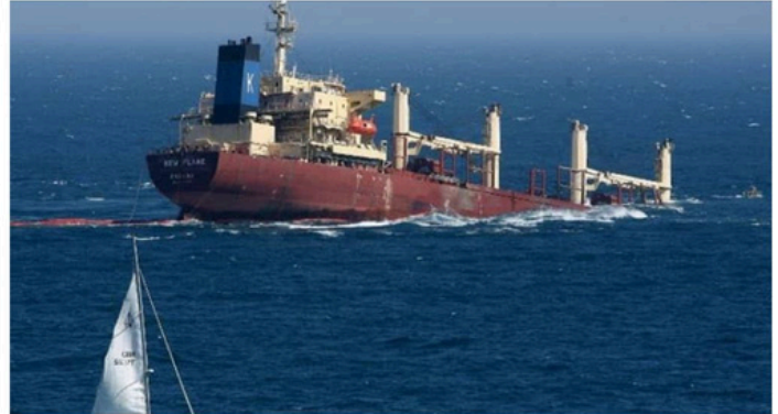
Fig. 3 Structural Failure of the New Flame
