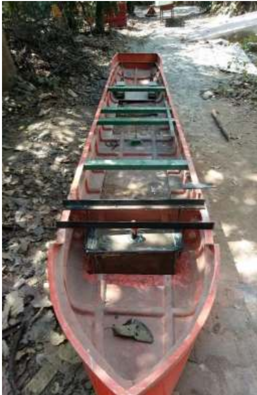
Fig. 5. Hull with cut sections for acrylic sheets
