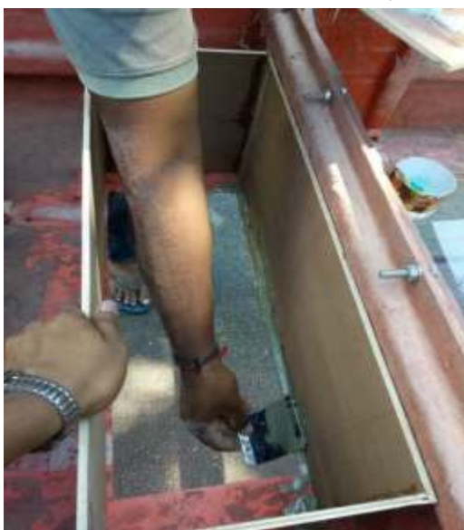
Fig. 6. Watertight chamber for the Injector unit
