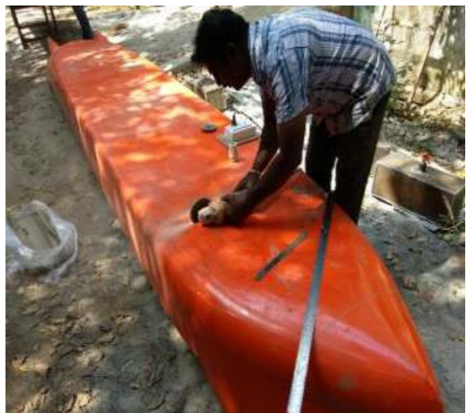
Fig. 4. Hull Cutting for the Injector Unit
