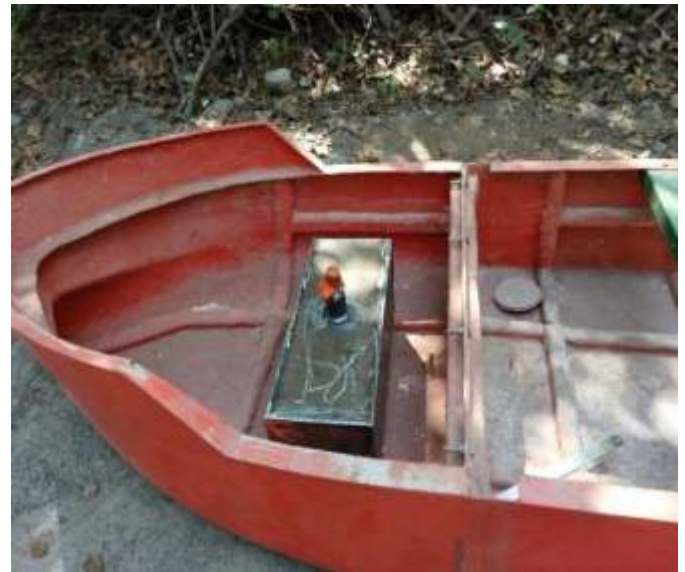
Fig.3. Location of Injector Unit, Placed at the Front
