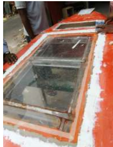
Fig. 11. Strengthening of acrylic sheet at bottom using putti and adhesives
