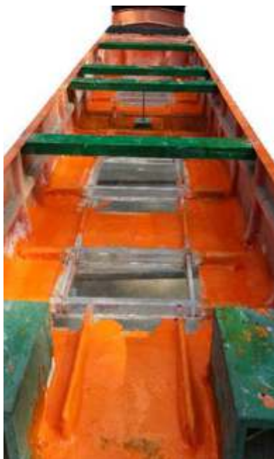
Fig. 10. Acrylic sheets placed for the visualization of flow
