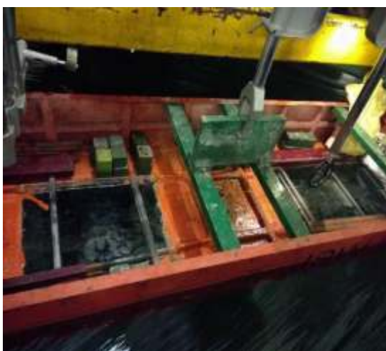
Fig. 13. Model with Ballast weights attached to towing tank
